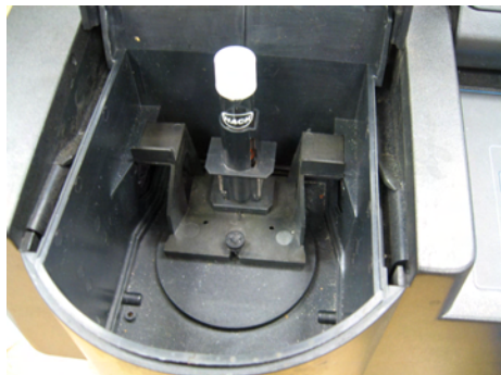
Figure: Insert tube into cell holder
