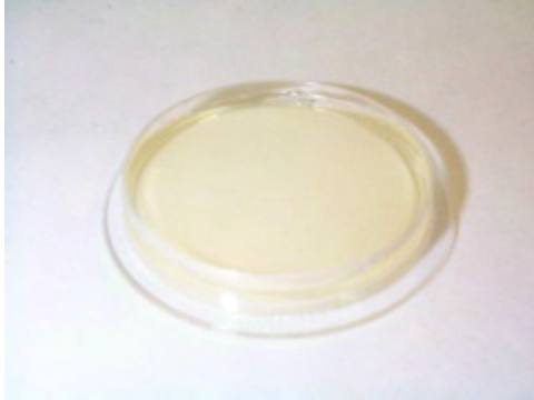
Figure: Sterility is checked by adding 5 ml TSB, incubating and checking for growth.
