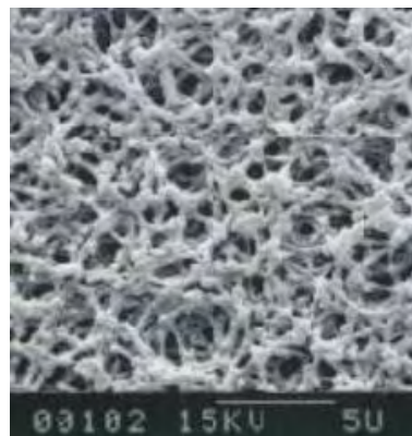
Figure: Notice the different size pores in this nominal filter. The tortuous path through the filter will catch most but some particles will manage to get through.
