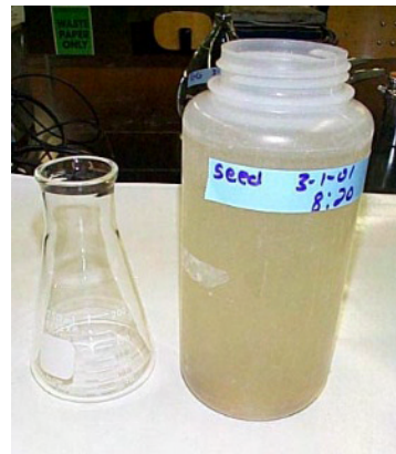
Figure 6: Settleable solids allowed to settle at least 1 and up to 36 hours
