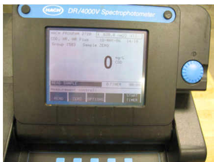
Figure: Zero the spectrophotometer using a reagent blank.
