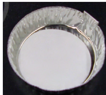
Figure: Weigh the dish and filter not just the filter.
