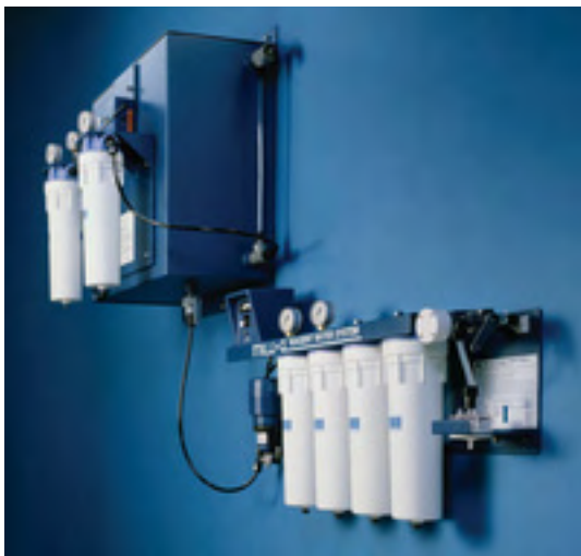
Figure: An example of a laboratory reagent grade water production system.
