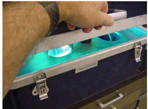
Figure: Sterilize for 2-3 minutes in UV sterilizer.
