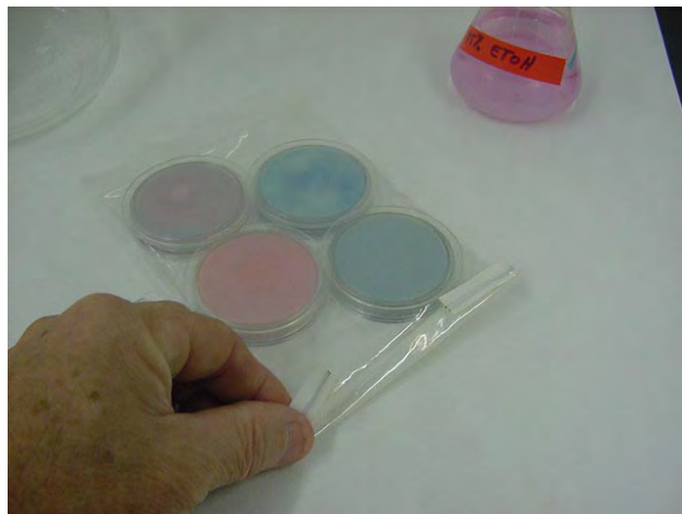
Figure: Squeeze out the air from the bag, roll the bag tightly, and then fold over the edges to seal the bag.
