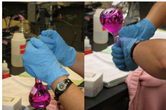
Figure: Cap and fill the volumetric flask, mix by inverting several times.
