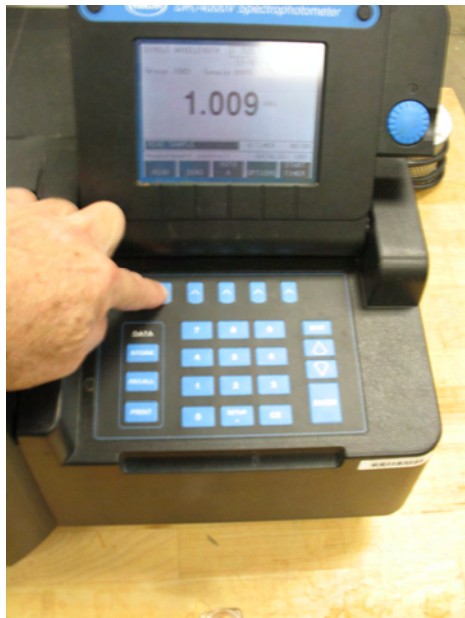
Figure: Press the read button to measure the concentration directly from the spectrophotometer.
