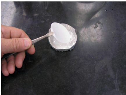
Figure: Always use forceps to handle the filter.
