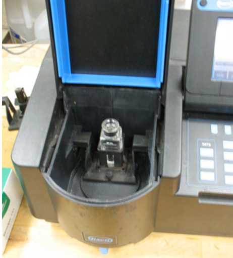
Figure: Place the reagent blank in the sample holder
