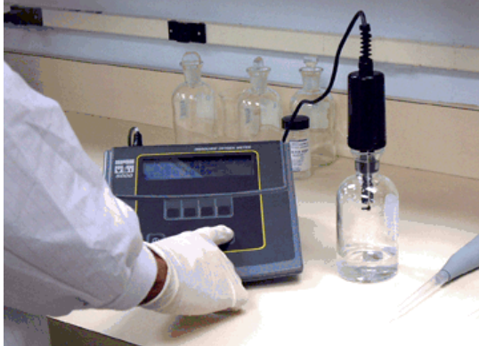
Figure: Laboratory calibration of DO meter with BOD probe
