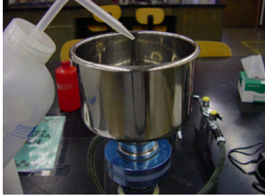
Figure: Rinse with DI water from top to bottom.
