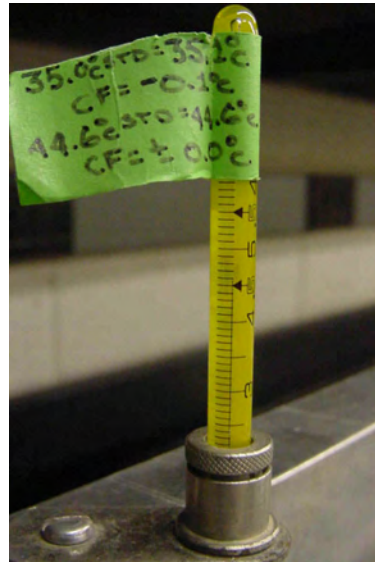
Figure: Notice the thermometer correction factor on the label.
