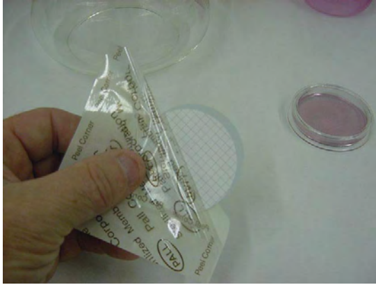
Figure: Carefully peel back the edges of the membrane filter. Sterile forceps can be used to help separate the filter from its blue backing. The blue backing is discarded.
