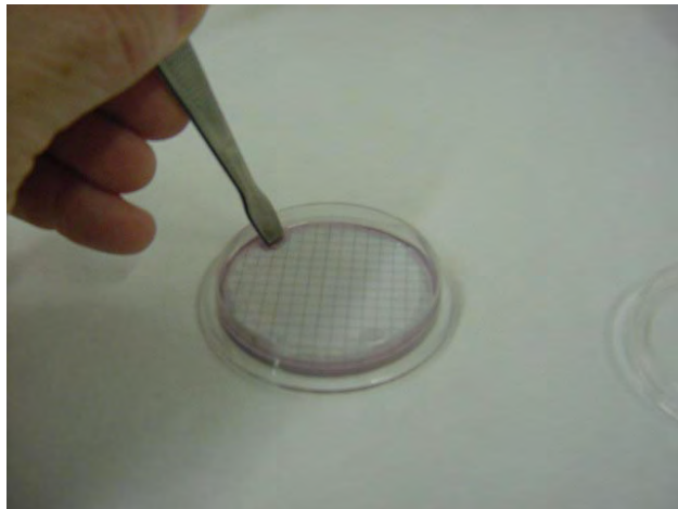
Figure: Gently secure the filter edges to the absorbent pad by running forceps around the perimeter of the Petri dish. Do not touch the area of the filter that contains bacteria.
