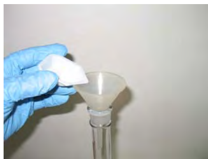
Figure: Use a funnel to transfer solids
