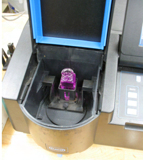
Figure: Place the sample into the sample cell holder, close the lid.
