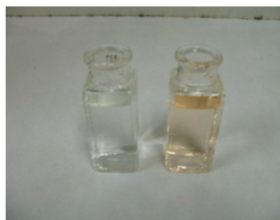
Figure: DI water blank vs. Reagent blank
