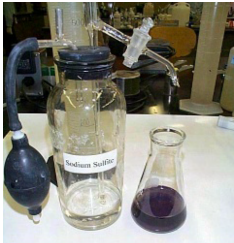
Blue color is titrated to clear using sodium sulfite
