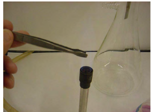
Figure: Do not overheat the tip of the forceps. The membrane will stick to hot forceps and tear.
